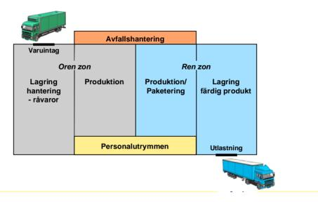
Figure 10. Example of a food plant with one section for unloading /goods reception and part of the production and one hygienic zone for processing, packaging, storage and transportation out from the plant /13/.
