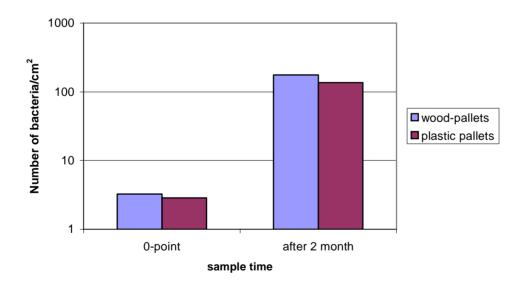
Figure 4. Bacterial count on wood pallets and plastic pallets (mean values) after 2 months in dry and warm environment.
