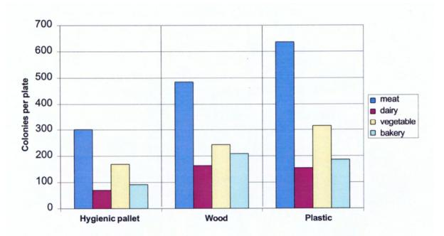
Figure 1 Bacterial count per plate - A comparison of hygiene pallets, wood pallets and plastic pallets in the meat, dairy, vegetable and bakery sector.
