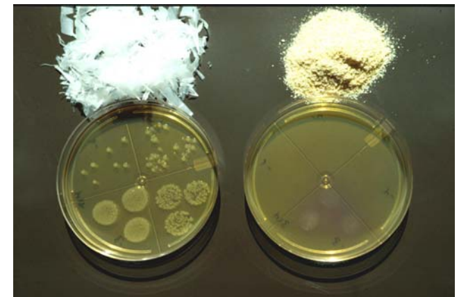
Comparison of the survival of Escherichia coli pIE639 on pine wood (right) and polyethylene (left) after 24 h
