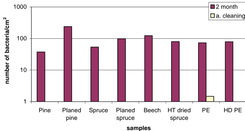
Figure 11. Effect of cleaning wood and plastic pallets using high pressure (180 bar) cold water treatment.
