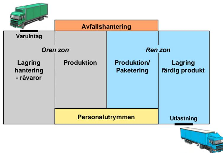
Figure 10. Example of a food plant with one section for unloading /goods reception and part of the production and one hygienic zone for processing, packaging, storage and transportation out from the plant /13/.
